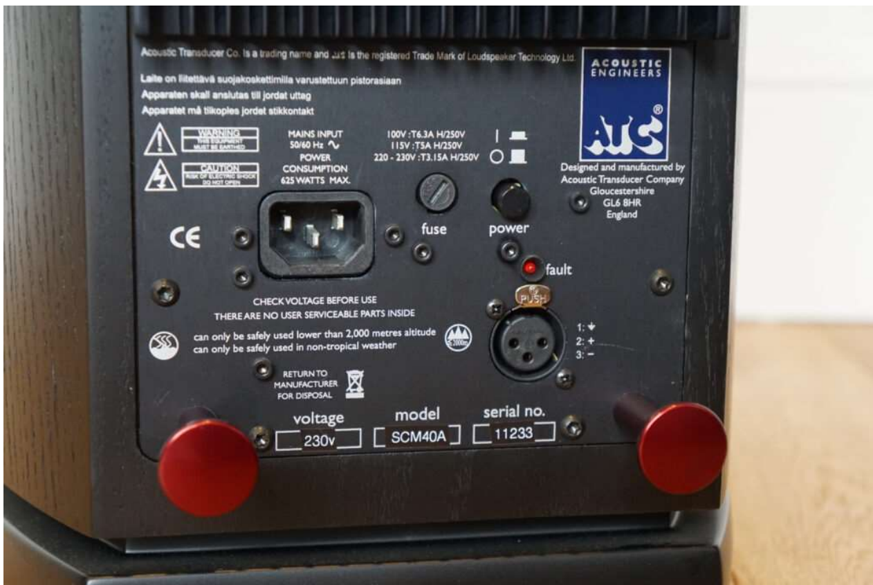
Rear electronics panel hosts on/off switch, mains and XLR inputs
